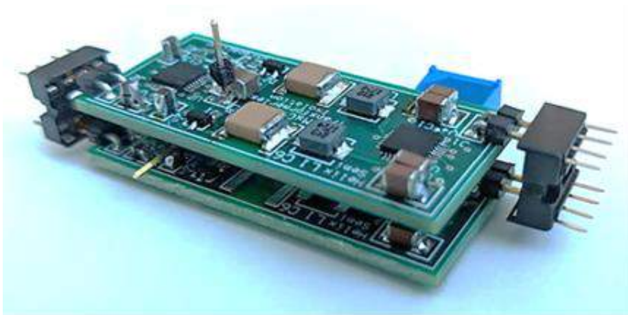
Figure 16: MxC 270 Output Current Sharing 20W 48V-to-12V TL EVM
