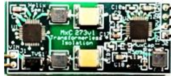
MxC 273-EB-C 5-10W 48VIN to Isolated \pm 12V & 5Vreg
