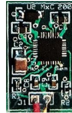
4x Voltage Boost + LED P/N: MxC 284-EB2-C
