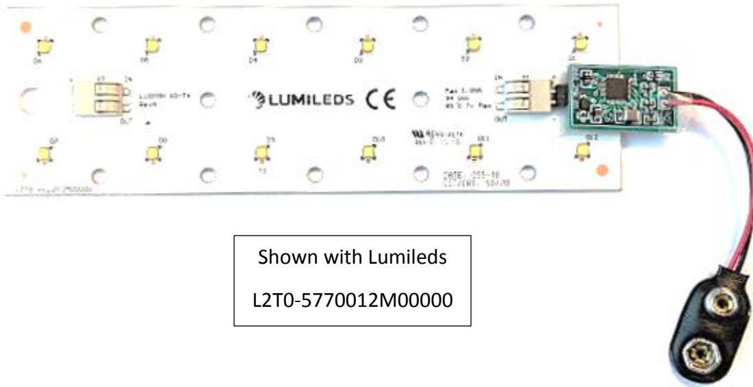
Figure 23: MxC 284 4x Voltage Boost with LED
